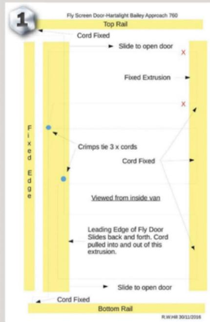
**1** Before removing the door, it helps to understand how it works. As the leading edge of the door is opened, all the cords are pulled up and down in the leading edge extrusion. There is a top drawstring that pulls the lower cords and a bottom drawstring that pulls the upper cords as the door is slid open
