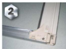
**2** Removing the door from the 'van is fairly straightforward. After removing the plastic bungs with a knife, unscrew the two self-tappers at the top corners and two self-tappers through the aluminium frame at the bottom
