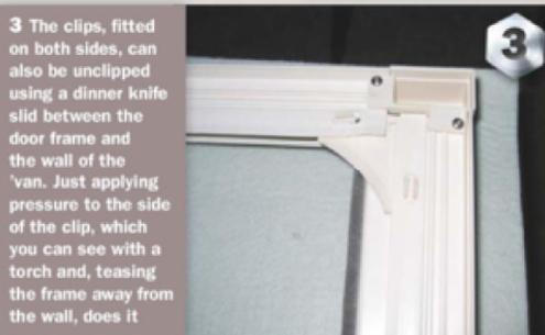
**3** The clips, fitted on both sides, can also be unclipped using a dinner knife slid between the door frame and the wall of the 'van. Just applying pressure to the side of the clip, which you can see with a torch and, teasing the frame away from the wall, does it
