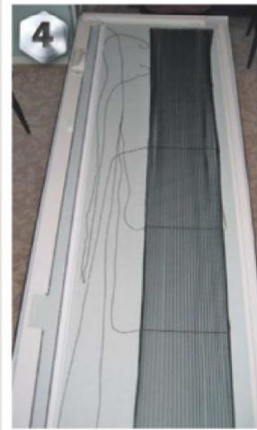
**4** Dismantling the door was done on the dining room table... much to the wife's dismay...but it was cold outside! There are self-tapping screws that need to be removed on the corners and plastic clips that hold the corners in place. These can be squeezed with pliers and the parts teased apart using a wide, flat screwdriver. Eventually, you will end up with the frame in four parts
