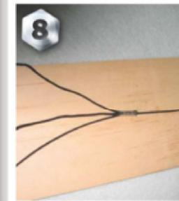
**8** I used the original lengths of broken cord to determine the length of my new loop and make sure that both ends were exactly in the right place for joining to the main cord. I then glued all three pieces of cord after scraping with a loose Stanley knife blade (carefully!) so that they were abraded. I used the open crimp to clamp them all together and then, after they had dried, dowsed the crimp in Super Glue to seal it
